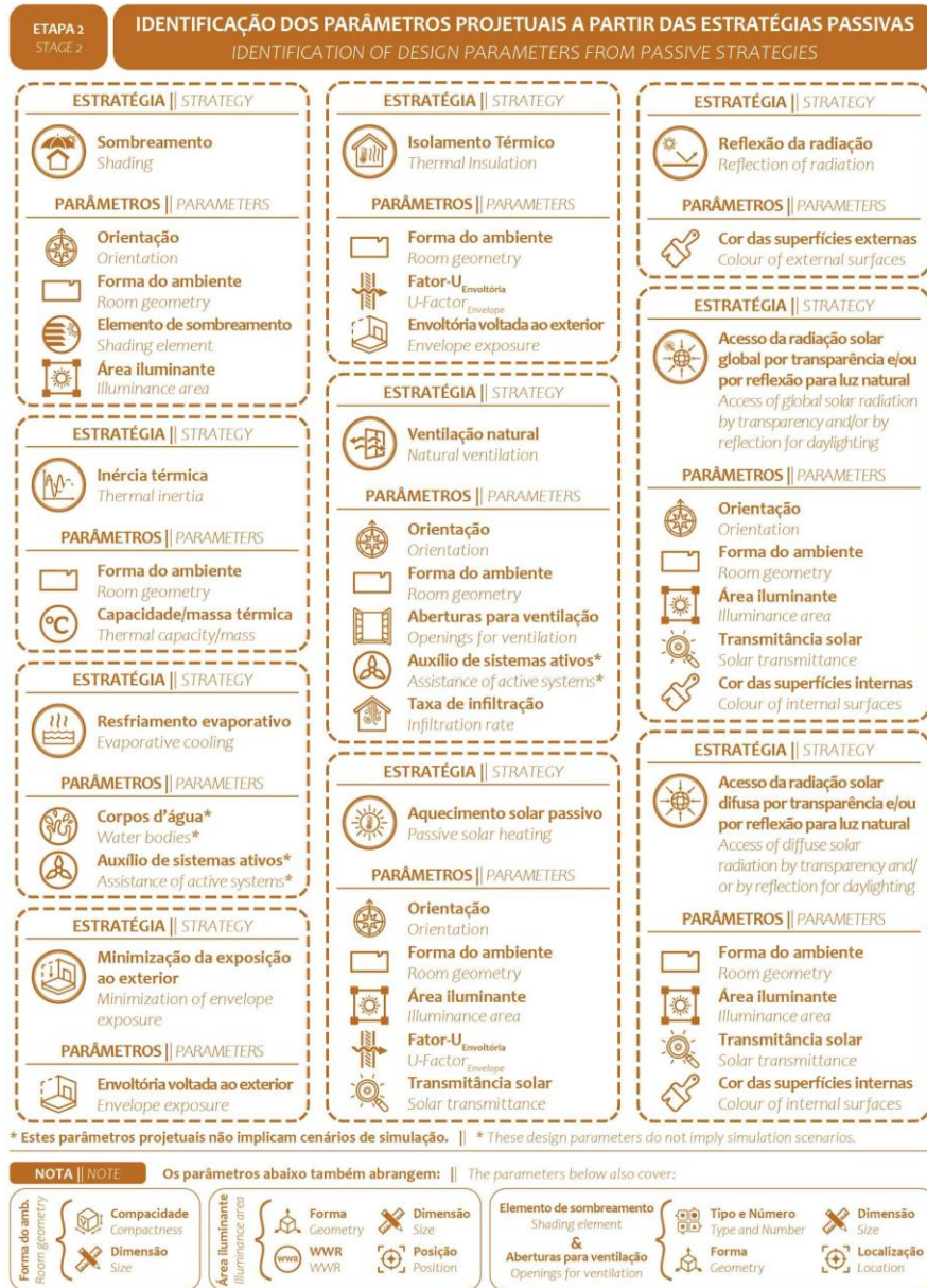
Figure 4 - Stage 2: Elaboration of the Base-Case, including the Identification of Design Parameters, the Elaboration of the Base-Cases themselves and of Alternative Scenarios, from the selection of passive strategies done in the previous stage. Source: the authors.
