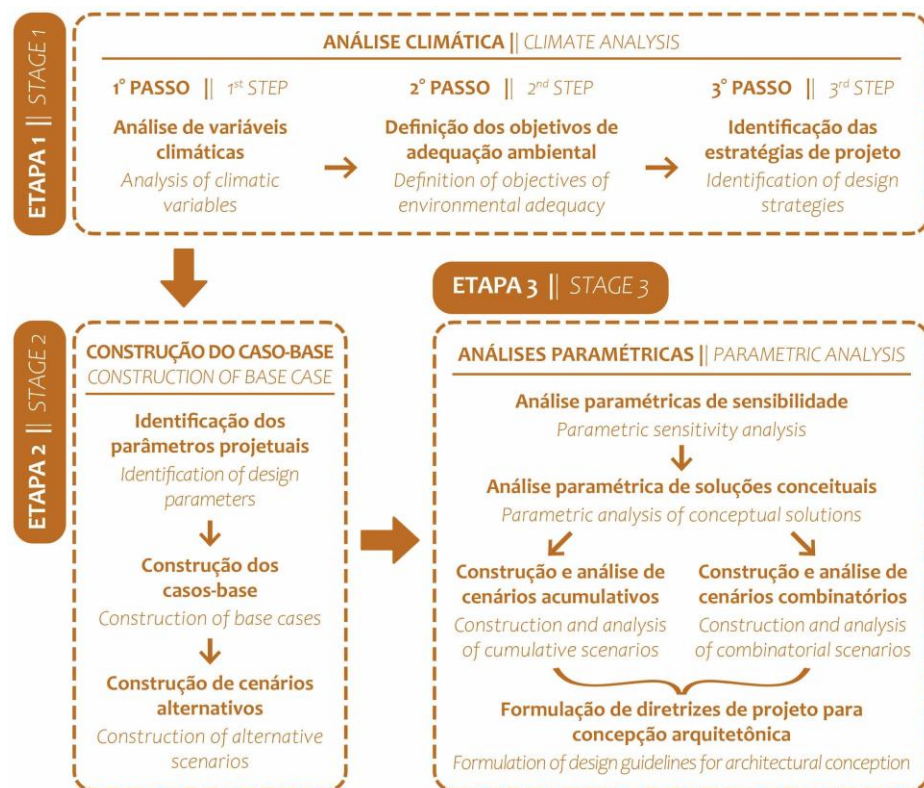
Figure 1 - Flowchart of the general stages of the methodological proposal for the insertion of environmental adequacy analytical procedures in the stage of architectural conception. Source: The authors.
