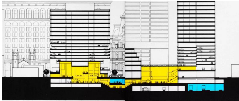
Figure 4. Section on Market Street. Adaptation of various movement systems. (Design of Cities, pp. 290-291)
